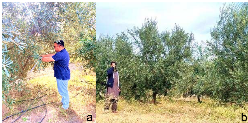
Figure 1. Measuring tree diameter with Caliper (a) and height of stems with Vertex Hypsometer (b).
