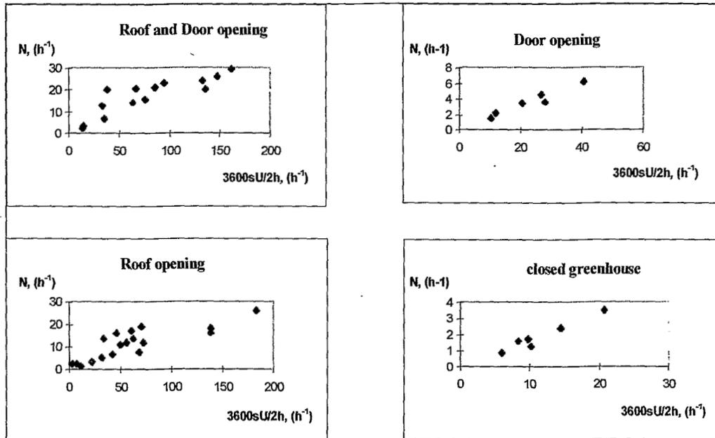
**Figure 3.  $N$  Versus  $(3600sU/2h)$  for roof, door, roof and door openings in the closed greenhouse**
