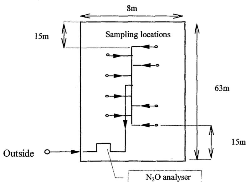
**Figure 2. Scheme of the tracer gas measurements. The  $N_2O$  analyzer aspirates the air from 8 positions equally distributed over the greenhouse and located at a height of 2m.**
