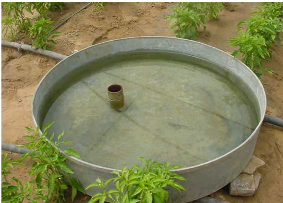
Fig. 3. Class A pan evaporation for measuring evaporation E_{pan} in greenhouse
