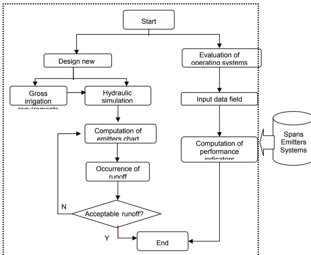
Fig. 1 Conceptual structure of the model DEPIVOT with indication of input data from a database
