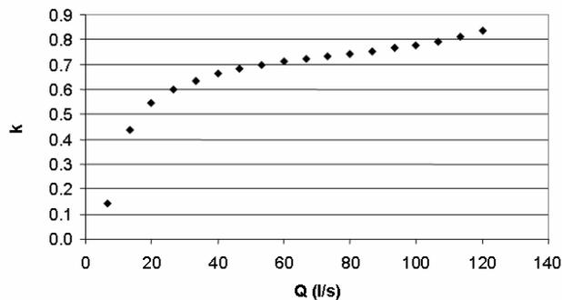
Fig. 4. Evolution of the calibration coefficient “k” with discharge.
