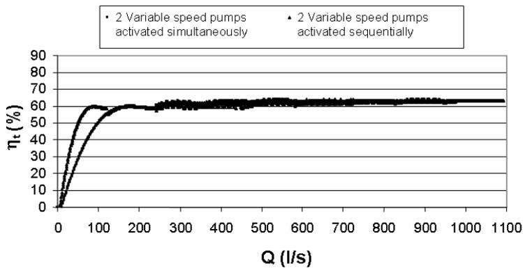
Fig. 8. Comparison between efficiency curves considering an activation of the variable speed pumps in a sequentially and simultaneously way.
