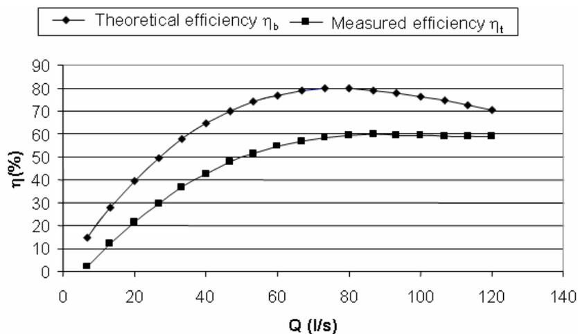
Fig. 3. Comparison between theoretical and measured efficiency curves of the variable speed pumps.
