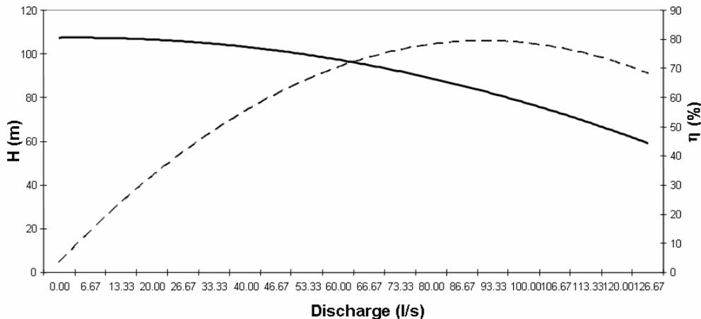
Fig. 1. Characteristic curves Q-H and Q- $\eta$  of the pumps
