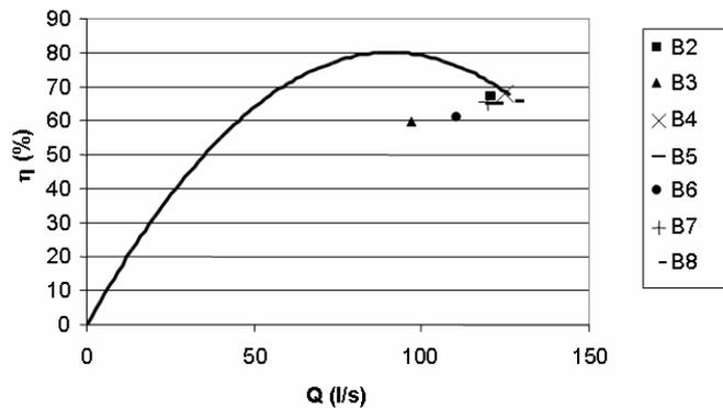
Fig. 5. Measured working points of the fix pumps and theoretical Q-H curve.
