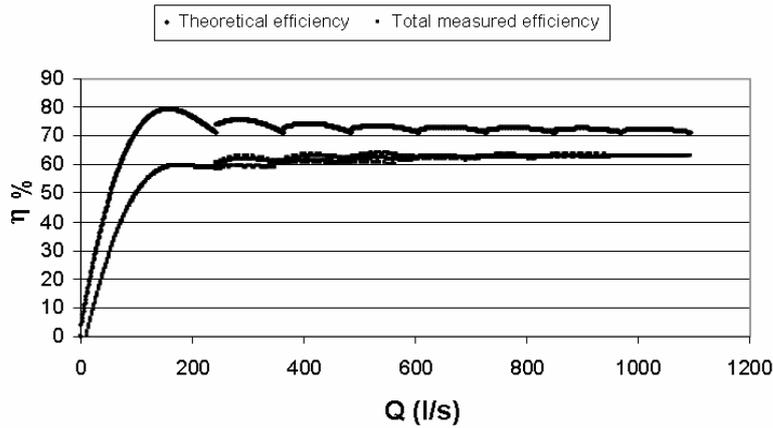
Fig. 7. Theoretical and measured efficiency for different discharges.
