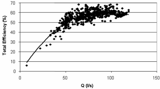
Fig. 2. Measured efficiency curve of the variable speed pumps
