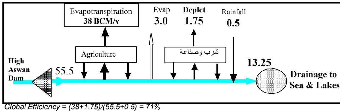
Fig 5. Schematic Diagram for Water Balance of Nile System in Egypt (Source: Allam, 2000)
