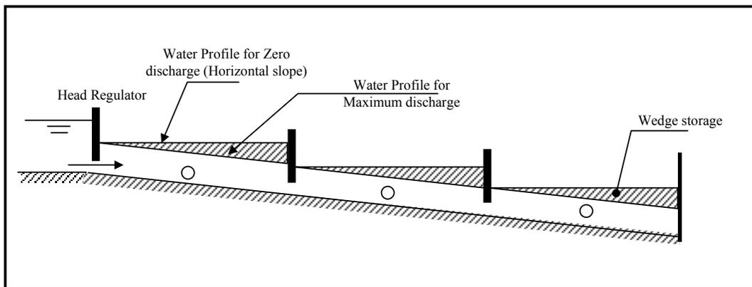
Fig. 4. Remodelling of Canal Storage
