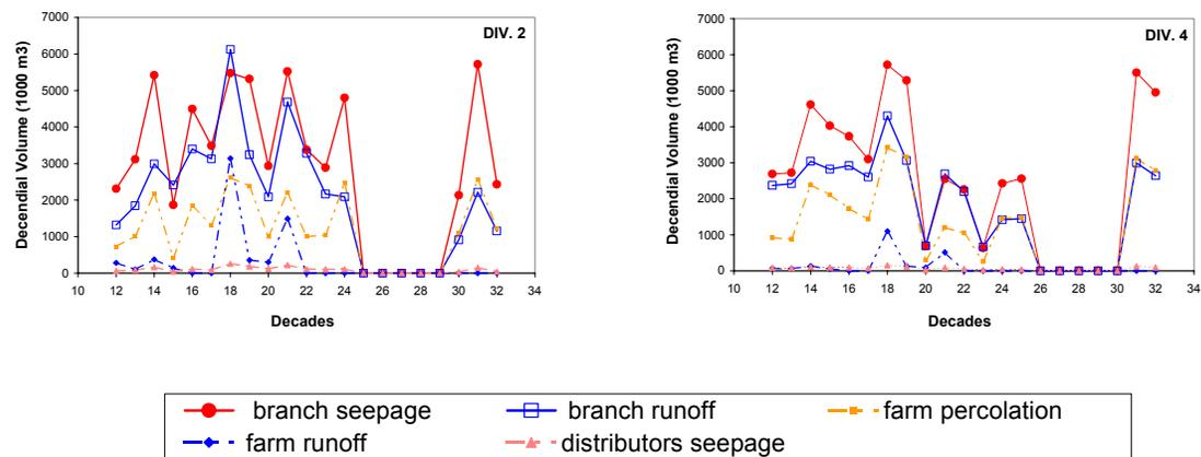
Fig. 7. Simulated seepage and runoff in branch and sub-branch canals, compared with percolation and runoff at farm level, and seepage in the distributors for Division 2 and 4.
