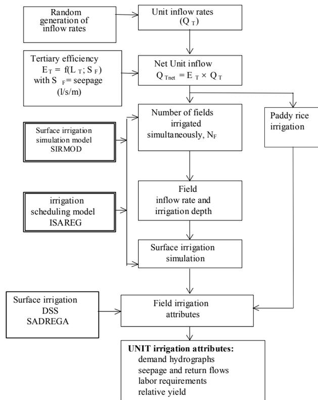
Fig. 4. Schema of the demand and delivery simulation at the unit scale.
