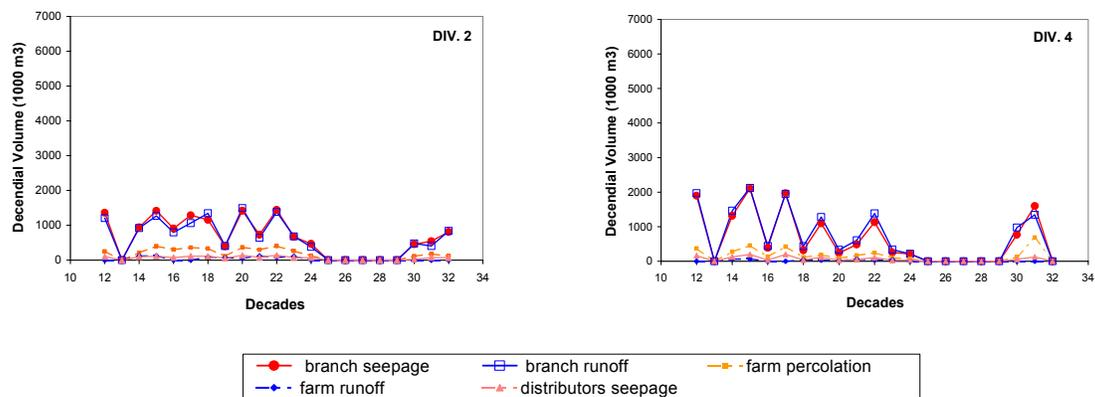
Fig. 9. Simulated branch canal seepage and runoff, distributors seepage, and farm percolation and runoff for Divisions 2 and 4.
