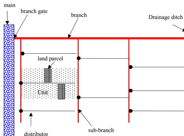
Fig. 2. Schematic representation of a distribution sub-sector network.
