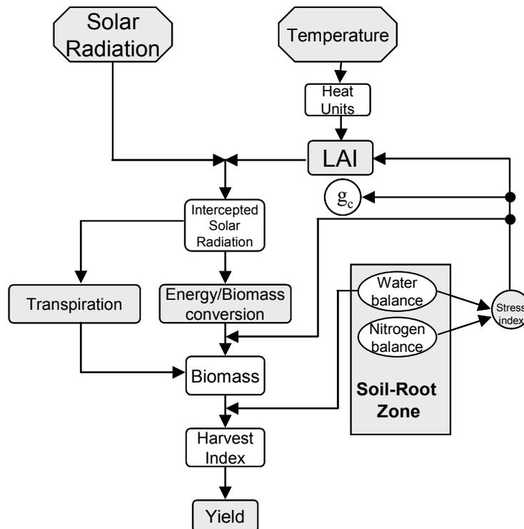
Figure 7. Schematic diagram of the relationships among the variables influencing growth and productivity in the crop model
