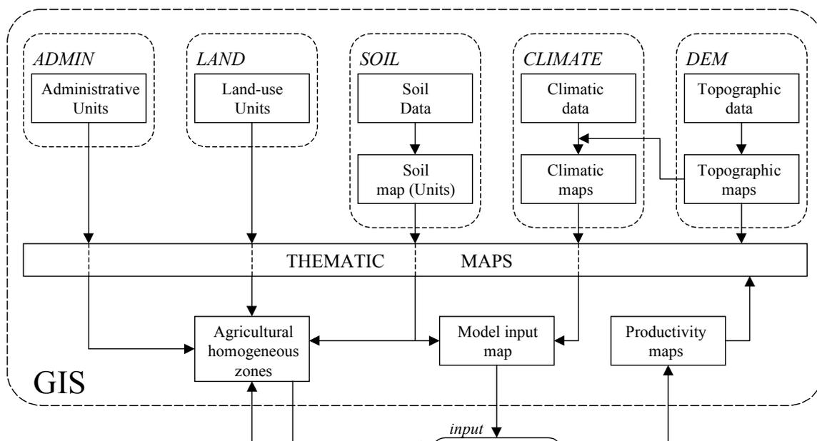
Figure 1. Schematic structure of the ACLA-2 information system and flowchart of main operations.
