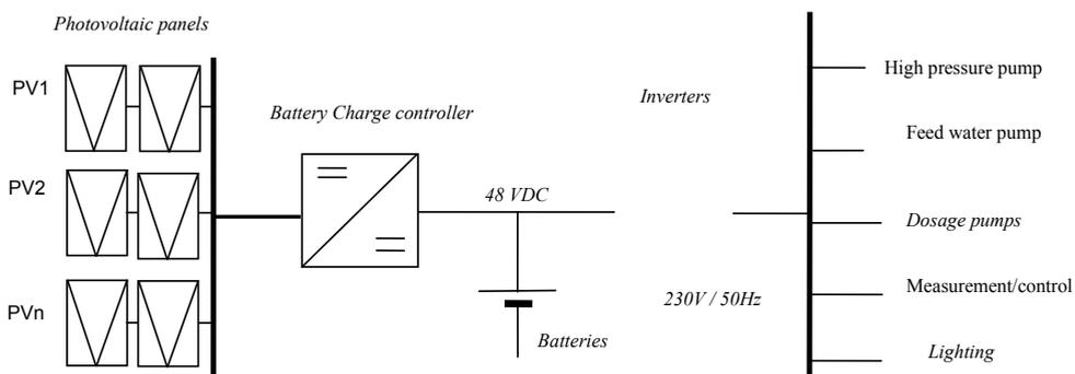
**Figure 1. Schematic diagram of the PV plant.**
