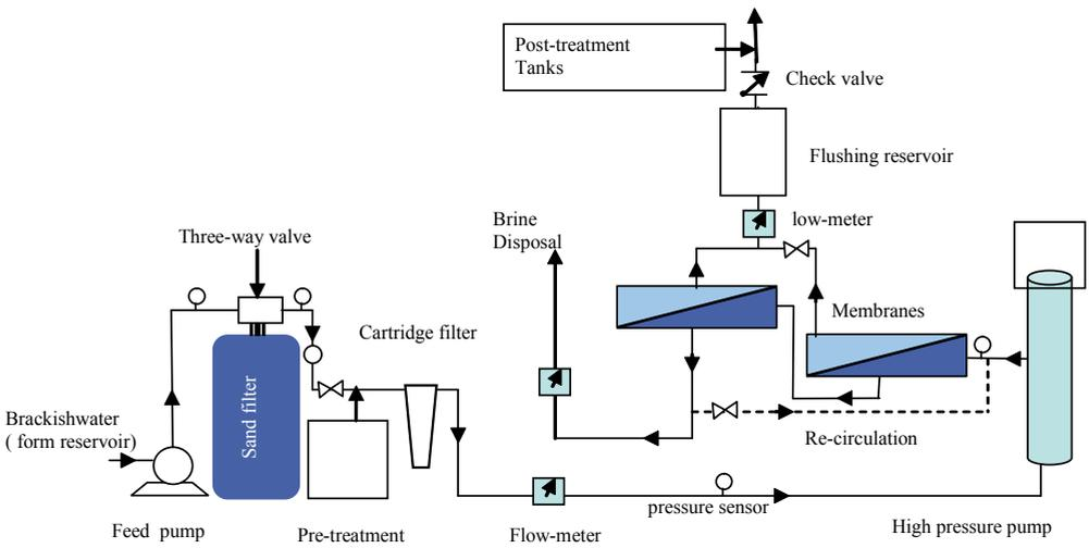
Figure 2. Schematic diagram of the RO plant.
