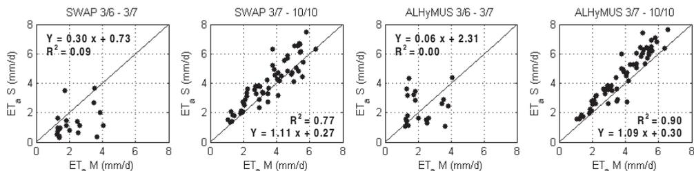
Figure 1. Evapotranspiration: measured values by EC technique ( $ET_a M$ ) vs. simulated ( $ET_a S$ ) by the two models using the PTFs of Rawls and Brakensiek (1989); periods 3/6/2006 - 3/7/2006 and 3/7/2006 - 10/10/2006.
