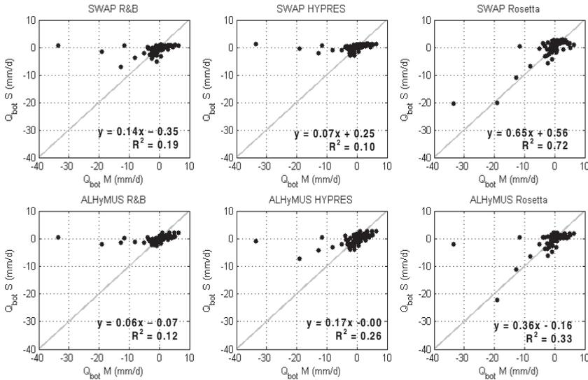
Figure 3. Bottom flux: measured values ( $Q_{bot} M$ ) and simulated ( $Q_{bot} S$ ) by the two models implemented with the different set of soil parameters.
