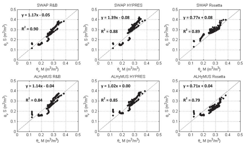
Figure 2. Soil moisture content in the root zone: measured values ( $\theta_v M$ ) vs simulated ( $\theta_v S$ ) by the two models implemented with the different sets of hydraulic parameters.
