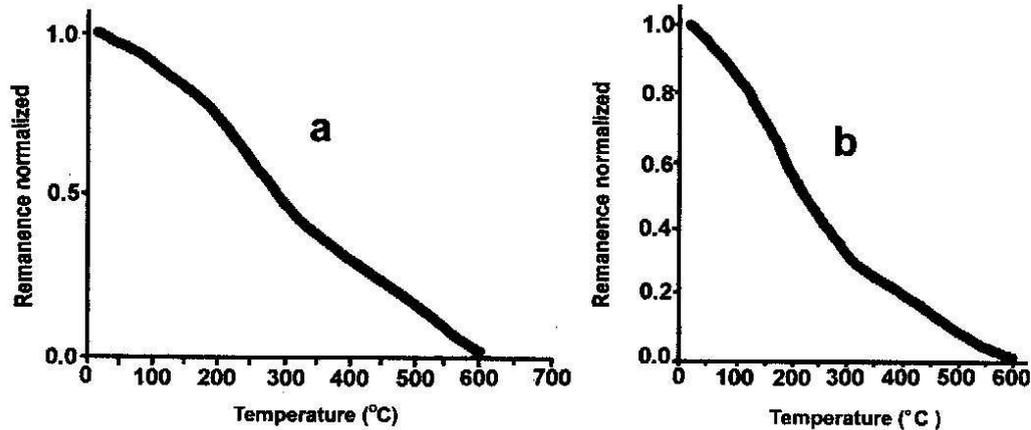
Figure 4. Temperature-dependent saturation remanence curves for terra rossa (a) and for upper horizon of alluvial sequence (b). Note similar shapes and different values for two soil types, indicating that magnetite is the main magnetic signal carrier.
