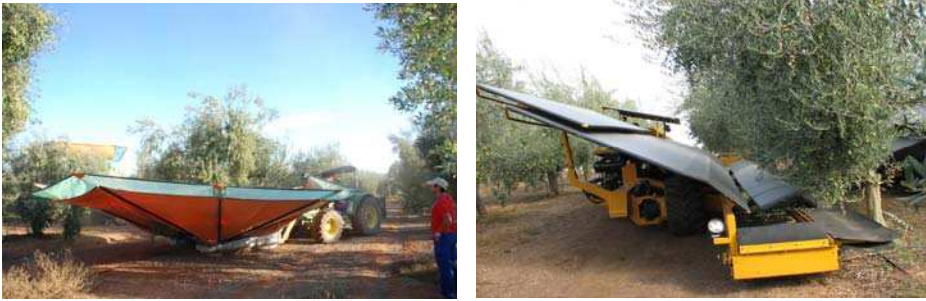
Fig. 9. Inverted umbrella trunk shaker (left) and side by side trunk shaker (right) in intensive olive orchard.
