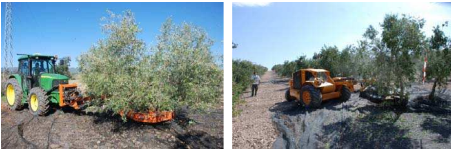
Fig. 7. Trunks shaker mounted on a tractor (left) and self-propelled trunk shaker (right).
