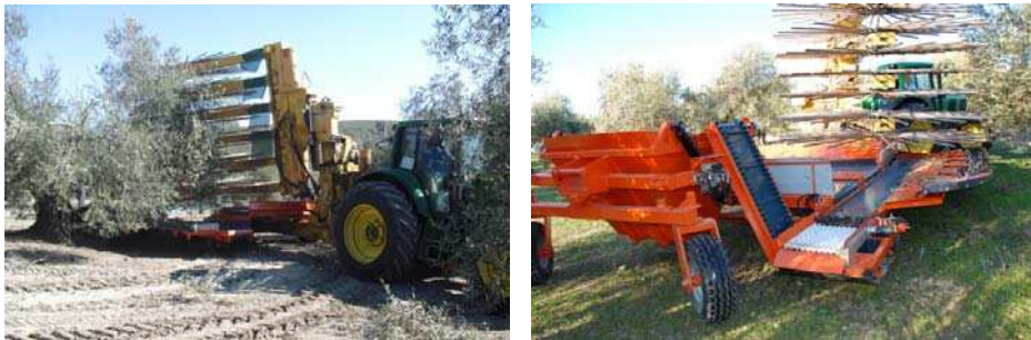
Fig. 8. Canopy shaker and catch frame adapted for traditional olive.
