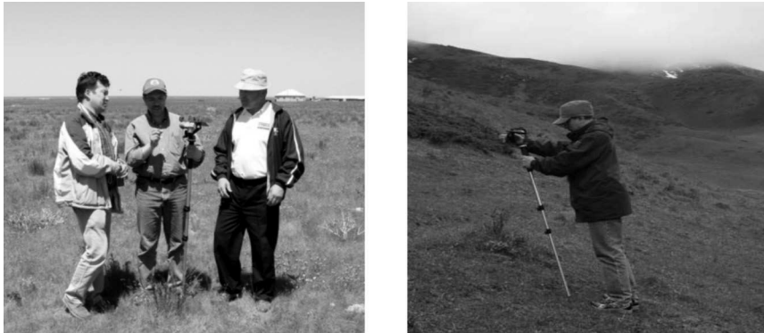
Fig. 2. The digital charting apparatus is being used in the field. Once the height of the monopod has been set it remains at that height for the sampling session. Because we work in the northern hemisphere, we usually point the camera due south which reduces shadow in the image.
