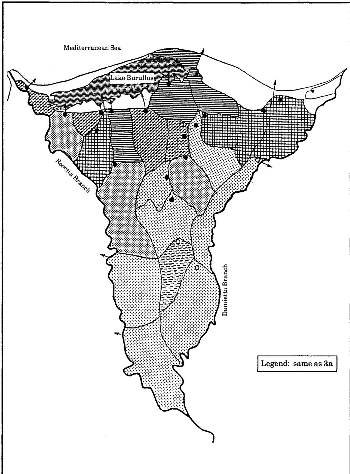
Figure 3c: Average salinity, 1986, of drainage water in the Middle Delta in g salts/m<sup>3</sup>
