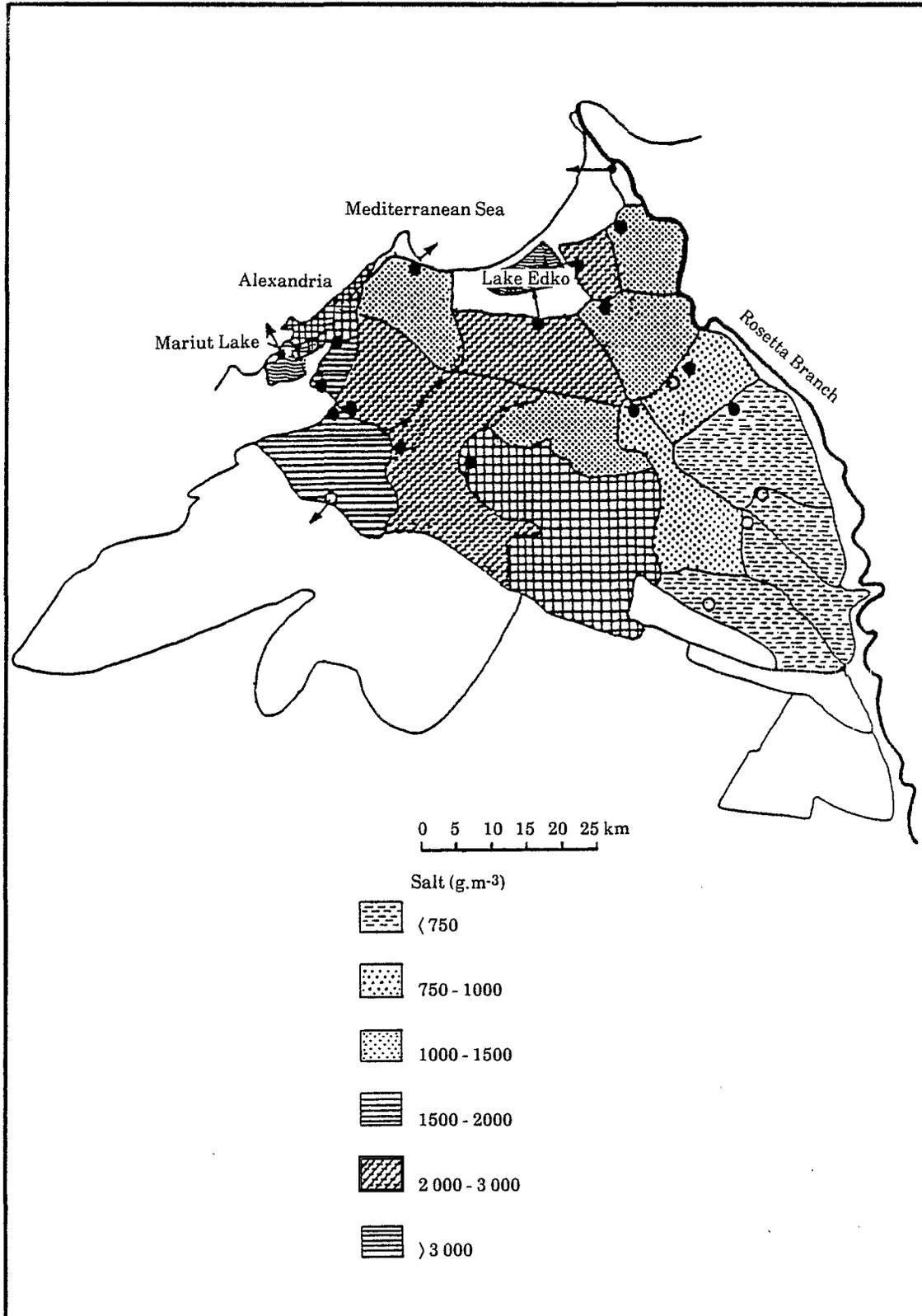
Figure 3b: Average salinity, 1986, of drainage water in the Middle Delta in g salts/m<sup>3</sup>
