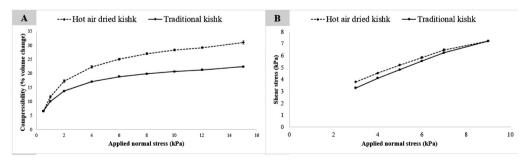
Fig. 1. Variation of kishk flow properties at different applied normal stress (A: powder compressibility test; B: shear test).
